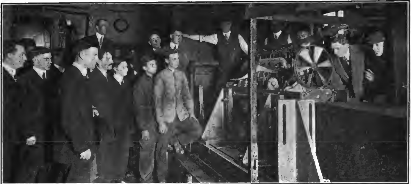
An interested gathering of engineers watched the conclusion of the 300-hour run of the Packard motor
